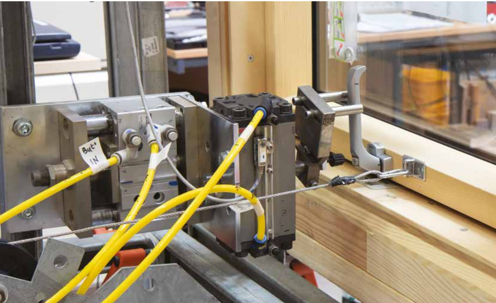
Window security test
