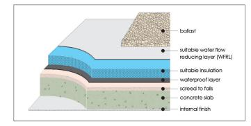
An inverted roof is quite simply where the waterproofing layer is installed below the insulation. Specifications for inverted roofs currently focus on several issues; in particular correct drainage and the corrections to calculated U values that result from cold rainwater seeping under the insulation, which carries heat away, and the effect of moisture on the insulation's conductivity.
