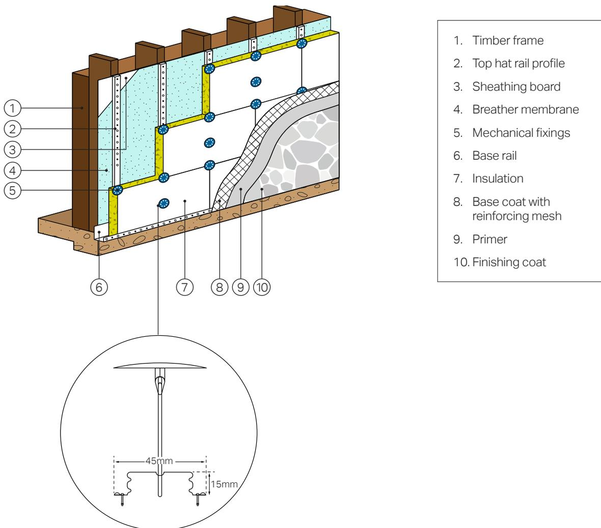
Figure 8 - Mechanically fixed EWS with vertical T-rail profiles
