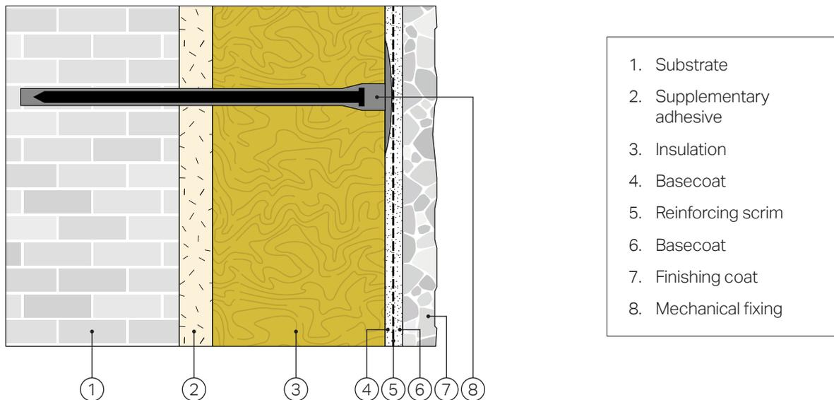
Figure 5 - Mechanically fixed EWIS (and extender washer), with supplementary adhesive
