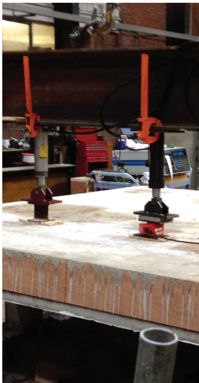
Bem and block floors tested to destruction
