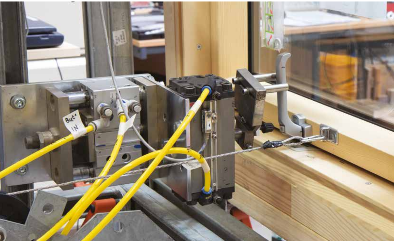
Window security test
