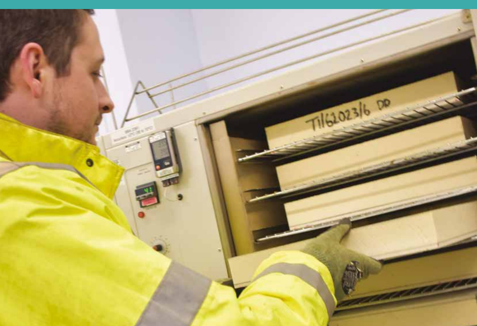
Thermal resistance facility
