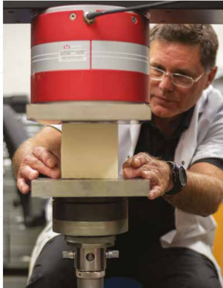
Compression resistance test
