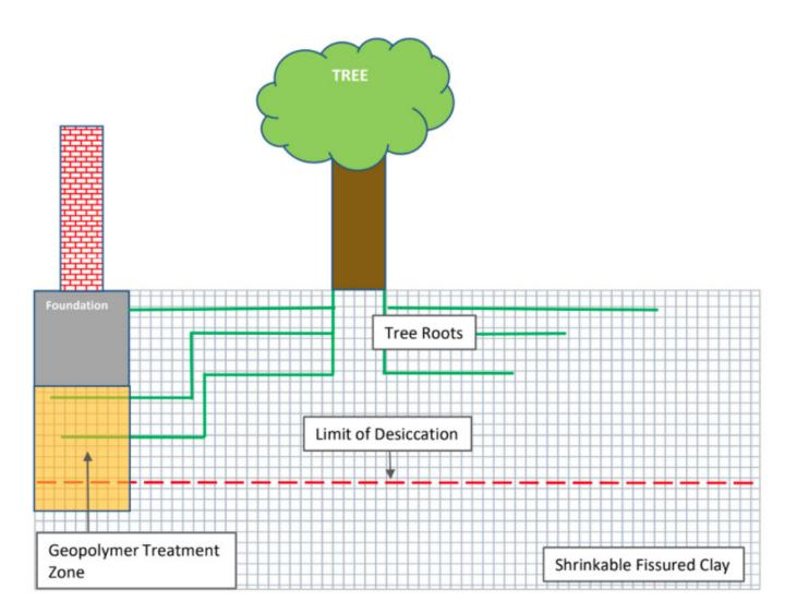
During the injection process the soil-structure interaction is monitored using laser level to an accuracy of +/- 0.5mm. A small positive reaction on the structure is required to confirm all the fissures have been filled with the expansive geopolymer.
